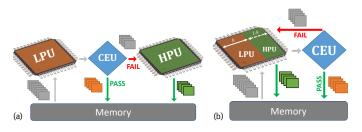
Fig. 5. CascadeCNN's architecture consisting of a low- and a high-precision unit, separated by a confidence evaluator acting on LPU's predictions: (a) Optimised for high-throughput, employing large batches and full device reconfiguration; (b) Throughput-latency co-optimised via resource sharing.
