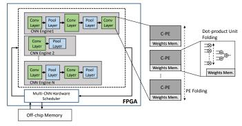
Fig. 7. Parallel architecture for multiple CNNs.
