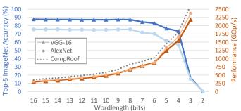
Fig. 6. Trade-off between precision, accuracy and performance of our novel CNN architecture (employed by both computational units of CascadeCNN), implemented on ZC706 FPGA. On both CNN models, CascadeCNN selects a 4-bit representation for the LPU and [6,8]-bit representation for the HPU depending on the user-specified error tolerance.
